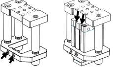
Install the front cover of Compliance Device. Align the holes on the front cover with the thread holes on the main bracket. The device must be seated flush against the bottom of the actuator air port protrusion. Apply Loctite 222 on the threads of two M6 flat head fasteners. Thread both fasteners through the front cover into the threaded bores on the main bracket. Torque both fasteners to 5Nm.
