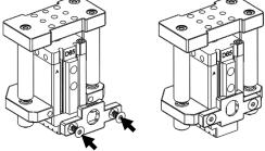
• Turn the tool to the other side and torque two M4 SHCS fasteners to 1Nm.
