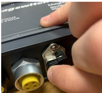
Figure 2 Rotary Cap Removal
