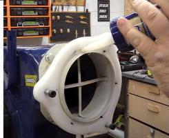
Fit seal over silicon in gap between the discharge port and collector plate.
