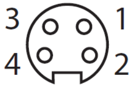
Cable Side: Pin Assignment 7/8", 4-pin, A-coded, Female Connector (socket-side) View
