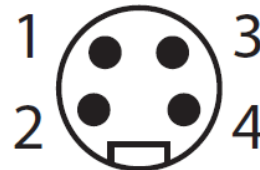
Tool side: Pin Assignment 7/8", 4-pin, A-coded, Male Connector (pin-side) View
