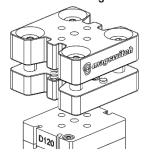
Insert 6mm Hex Driver through the center hole on top of Compliance Device. Thread and tighten the fastener through the bottom plate into the threaded bore on top of D120. Torque the fastener to 41Nm.
