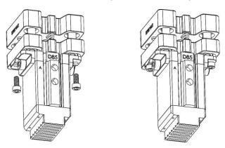
The installation of D85 Compliance Device is complete. There should be no visible gaps between the D85 tool and the Compliance Device.
