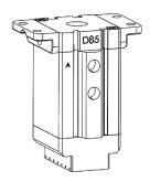
Apply Thread Locking Compound on the thread of M8 Socket Head fasteners. Thread and tighten the fasteners through the brackets into the threaded bore on sides of D85. Torque the fastener to 41Nm.
