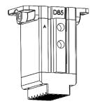
Insert two dowel pins into the dowel holes on the bottom of Compliance Device.
