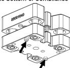
• Install the Compliance Device on top of D85. Align two dowel pins with the dowel holes on top of brackets. Insert dowel pins until the Compliance Device is flush against brackets and D85.
